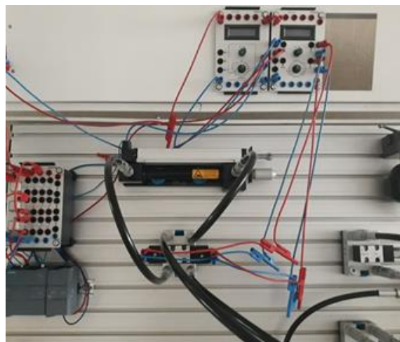
Figure 3. Implemented circuit for closed-loop control of proportional hydraulic valve with PLC
