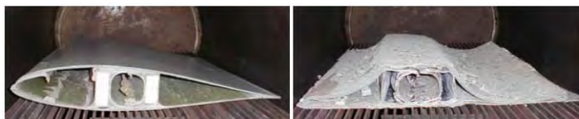
Wind Turbine Blade prior to pyrolysis Plastic is gasified – 55 % fiber is left
