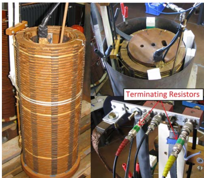
Fig. 3. Experimental setup; HV and LV winding (left); windings inside the outer cylinder (top right); connection cables with terminating resistors (bottom right).
