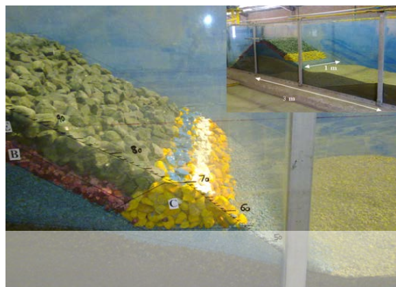
Fig. 1. Breakwater model (slope 1:0.66), side view.
