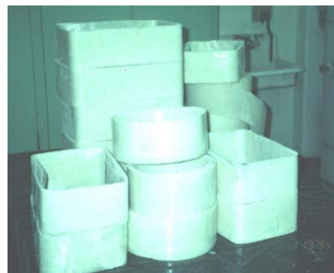
Fig. 4. FRP wraps (or straps) fabricated in the laboratory for the study.
