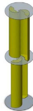
Figure 4. Savonius models for simulation, Where Paddle 1 [F 1 ] (b) Paddle 2 [F 2 ] (c) Paddle 3 [F 3 ] (d) Paddle 4 [F 4 ].
