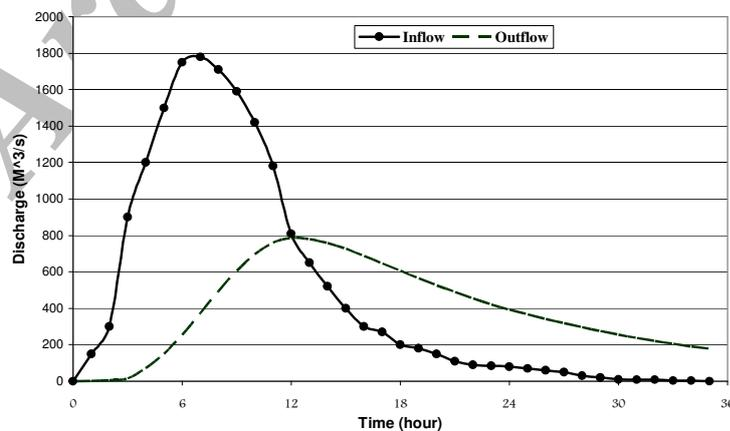
Figure 4. Inflow and outflow hydrograph during the flood.
