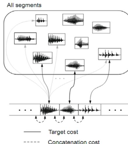
Fig. 1. General Scheme of Unit-Selection Synthesis [3]
