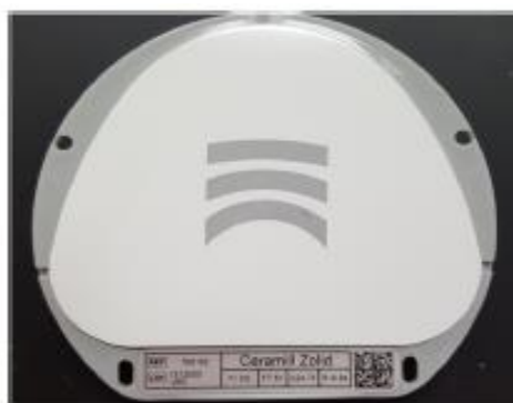
Figure 9. Presintered Zolid blocks
