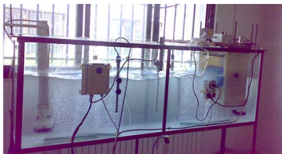
Fig. 1. The seawater containing tank equipped with instruments to simulate environmental conditions of recreational water in the southern coast of the Caspian Sea and used as a model microcosm.
