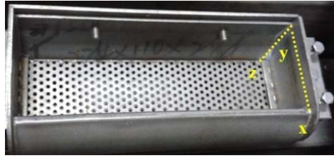
(a) Solder pot (Limits of level XYZ for solder fountain formation).
