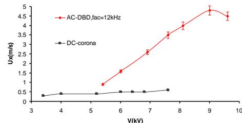
**Fig. 12. Tangential induced velocity by AC-DBD and corona plasma actuators in  $Y=0.3\text{mm}$  above the flat plate surface (nearest point to the wall where Pitot tube can be installed).**
