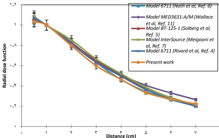
Figure 4. Comparison of radial dose function of the new IrSeed  $^{125}I$  source in plexiglass with data those for other  $^{125}I$  sources reported by Nath et al., Wallace et al., Solberg et al., and Migooni et al. [5,6,7,11]
