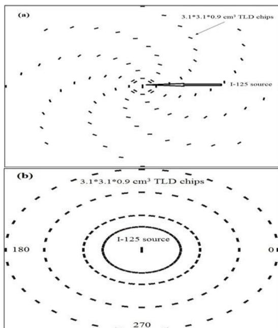
Figure 3. Schematic diagram of the plexiglass phantom design for measurement of (a) radial dose function and (b) anisotropy function using TLDs.
