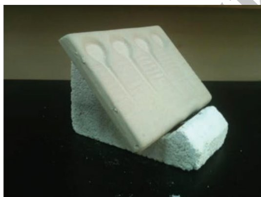
Fig. 3. Groove viscometer for measuring and comparing the viscosity of the samples.
