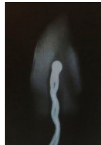
Figure 1. Position of the Tip of Thermocouple in the Pulp Chamber.
