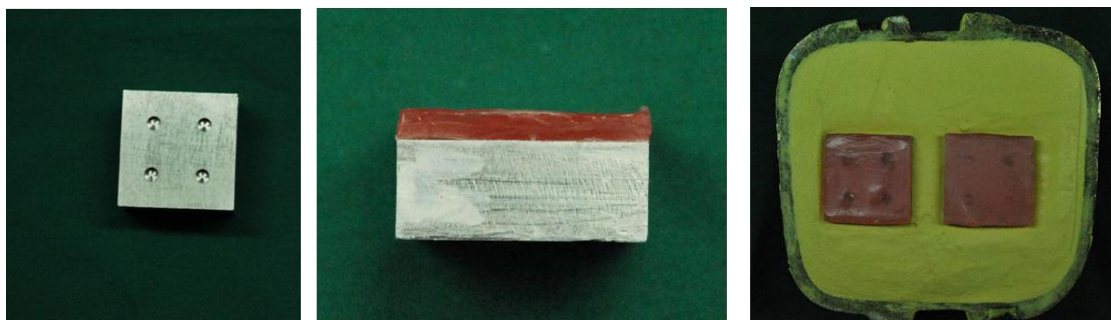
Fig 1. (a): Original specimen made from stainless steel, (b): Two layers of wax placed on stainless steel plates, (c): The plates embedded in a flask
