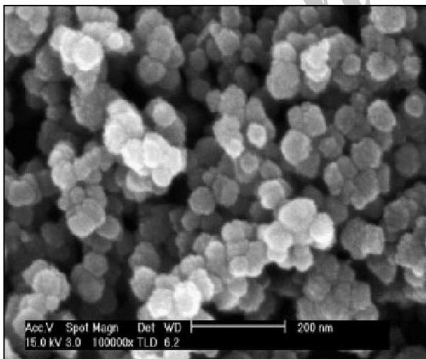
Fig. 1. SEM image of hydrophobic magnetic nanoparticles
