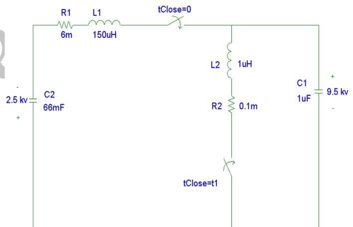
Fig. 2. Test circuit designed for testing 50 Hz breakers
