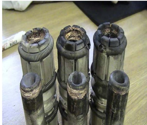
**Fig. 8. Failed specimen in CESI laboratory direct tests**
