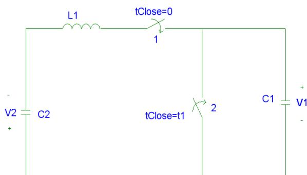
Fig. 1. Schematics of the proposed test circuit
