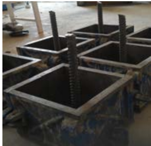
Figure 2. Details of reinforcement and mold
